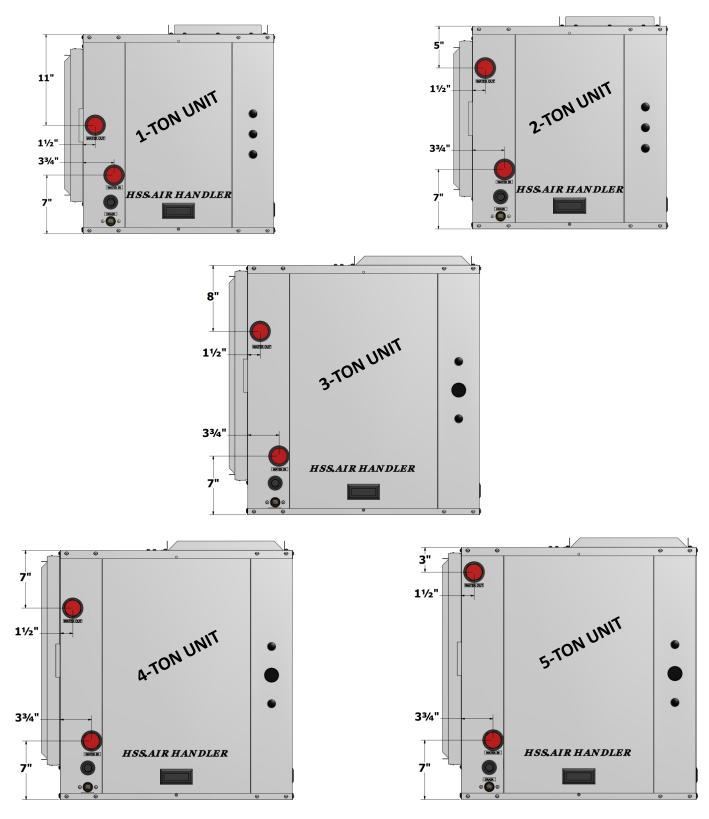
NOTE: Measurements are Listed in Inches NOTE: Distances Listed are Edge of Air Handler to Center of Swivel
